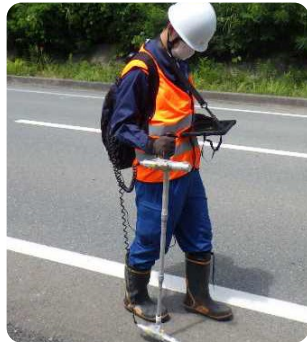
Post-decontamination walk-down monitoring
