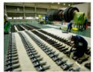
Diagnosing turbine blades by dismantling them
