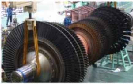
Taking out gas turbine for maintenance
