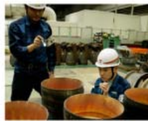
Visual inspection on gas turbine combustor
