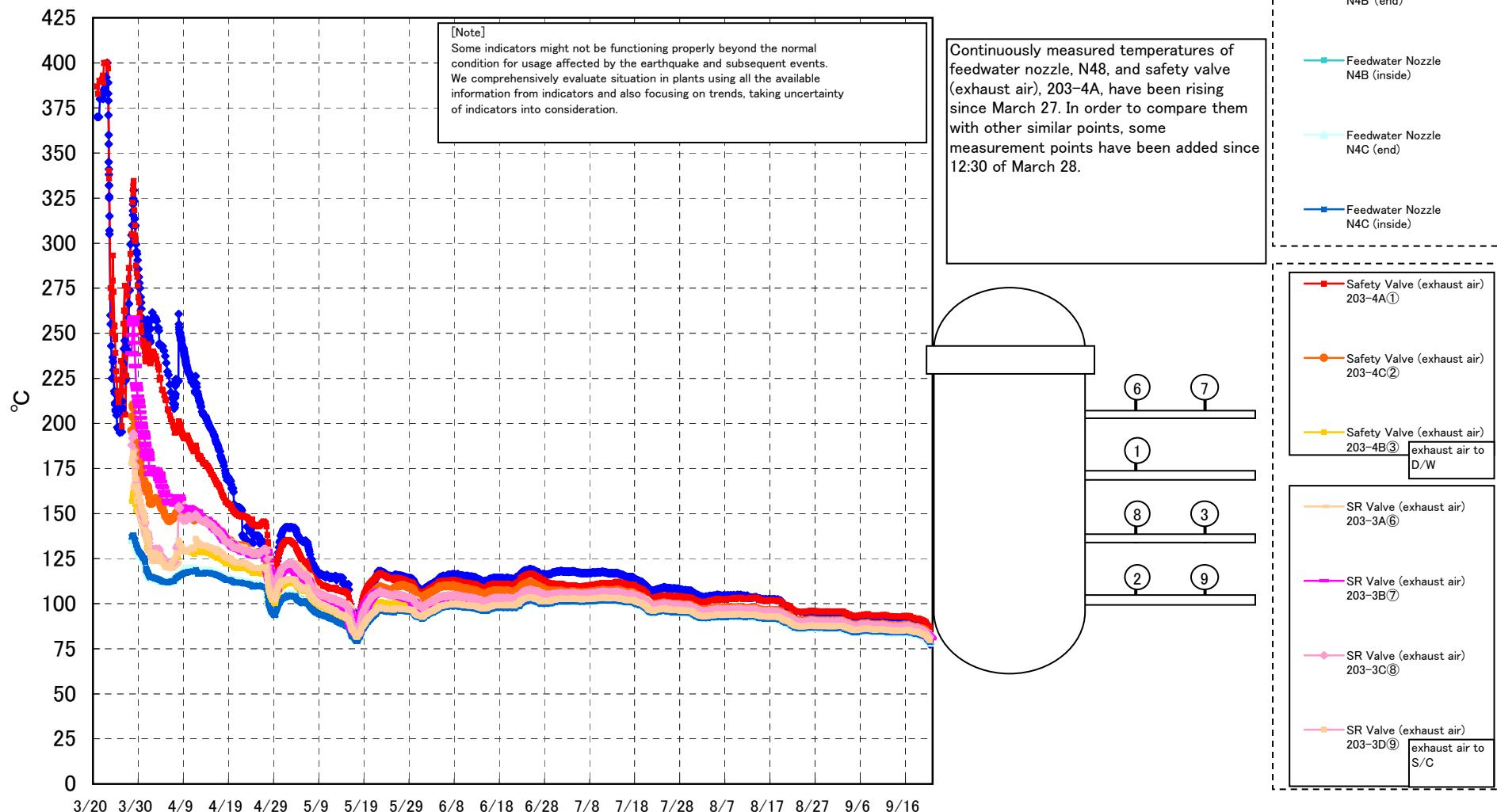
Fukushima Daiichi Nuclear Power Station Unit1 Parameters of Temperature
