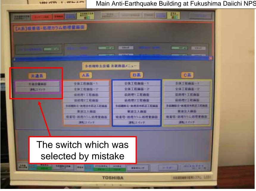
Multi-nuclide Removal Equipment Monitoring Panel in the Main Anti-Earthquake Building at Fukushima Daiichi NPS 共通帝スイッチ 多核種除去設備系 Common System The switch which should have been selected A系 Common Facility Screen 全体工程画面-1 Operation Switch 全体工程画面-2 前処理1工程画面 The switch which was 前処理2工程画面 selected by mistake 多核種除去·処理済水移送工程画面 薬液注入画面 吸着塔・処理カラム処理量画面 運転スイッチ
