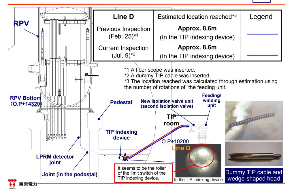
Dummy TIP cable head
