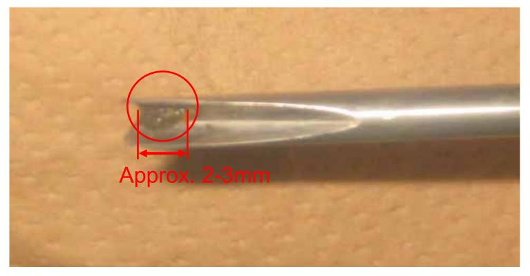
After the dummy TIP cable was pulled out, attached substances were found on the head.
