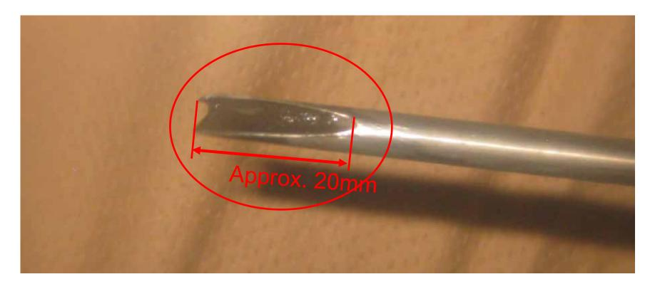
After the dummy TIP cable was pulled out, attached substances were found on the head.
