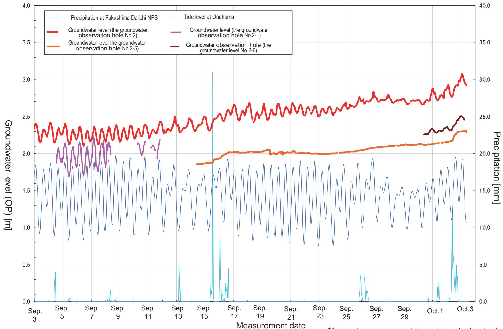
\*Automatic measurement through a water level indication
