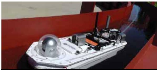
Surface boat: Travel test at factory
