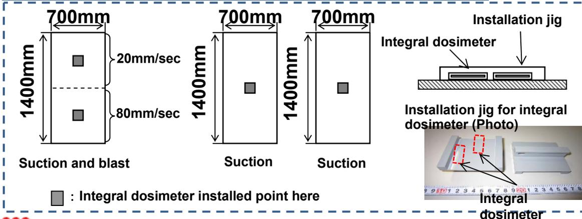
Blast decontamination processing (mock-up)
