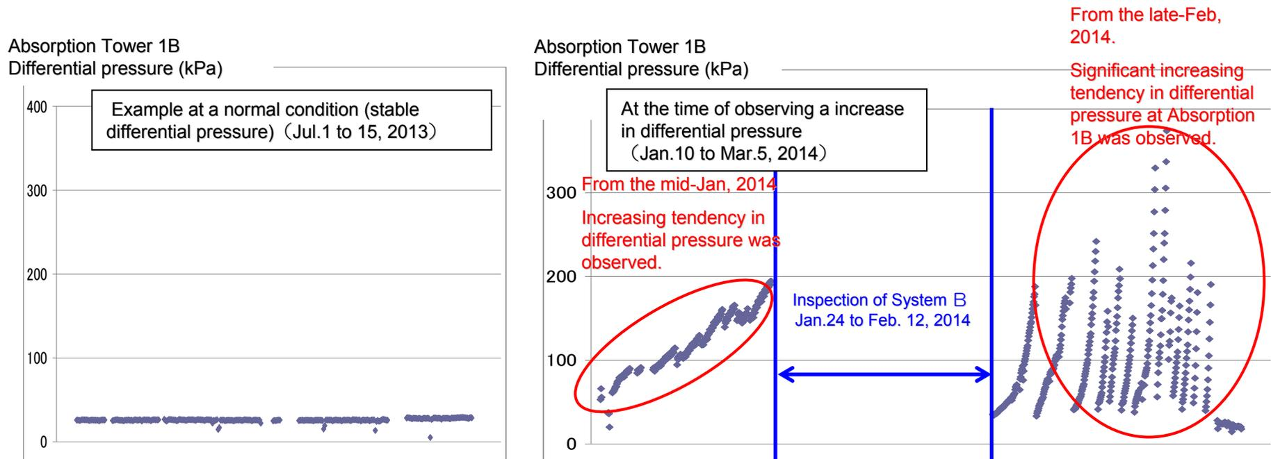
Over-time changes of differential pressure at Absorption tower 1B
