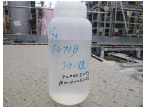
← No white sediment was found in the blow water taken from the vent pipe (the stagnation part) at the exit of System B.
