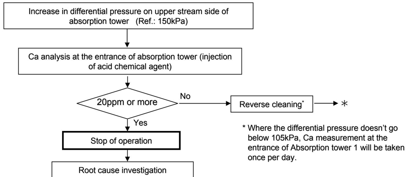
Judgment flow for implementation of reverse cleaning on the upper stream side of absorption tower
