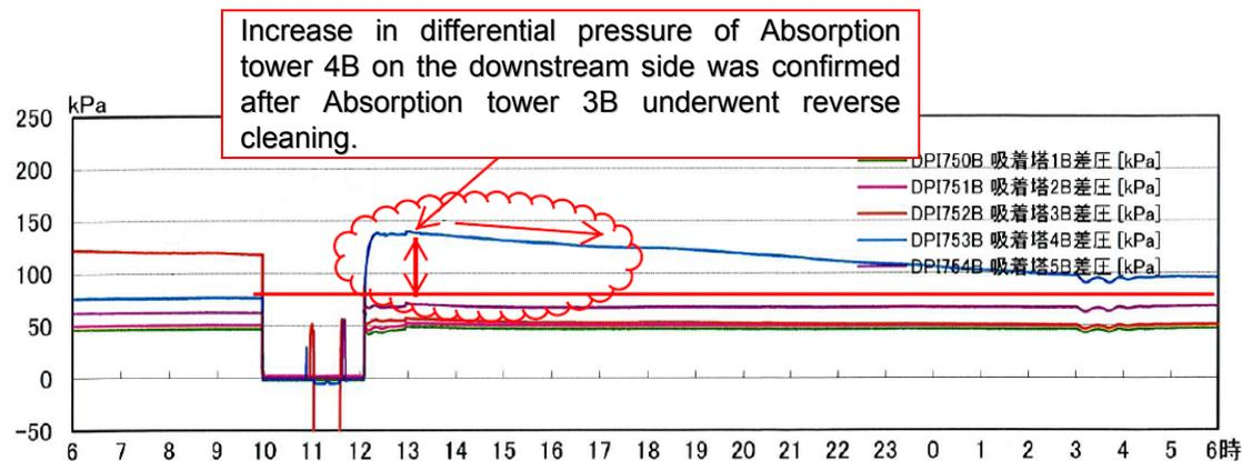
Example of differential pressure increase after reverse cleaning absorption tower
