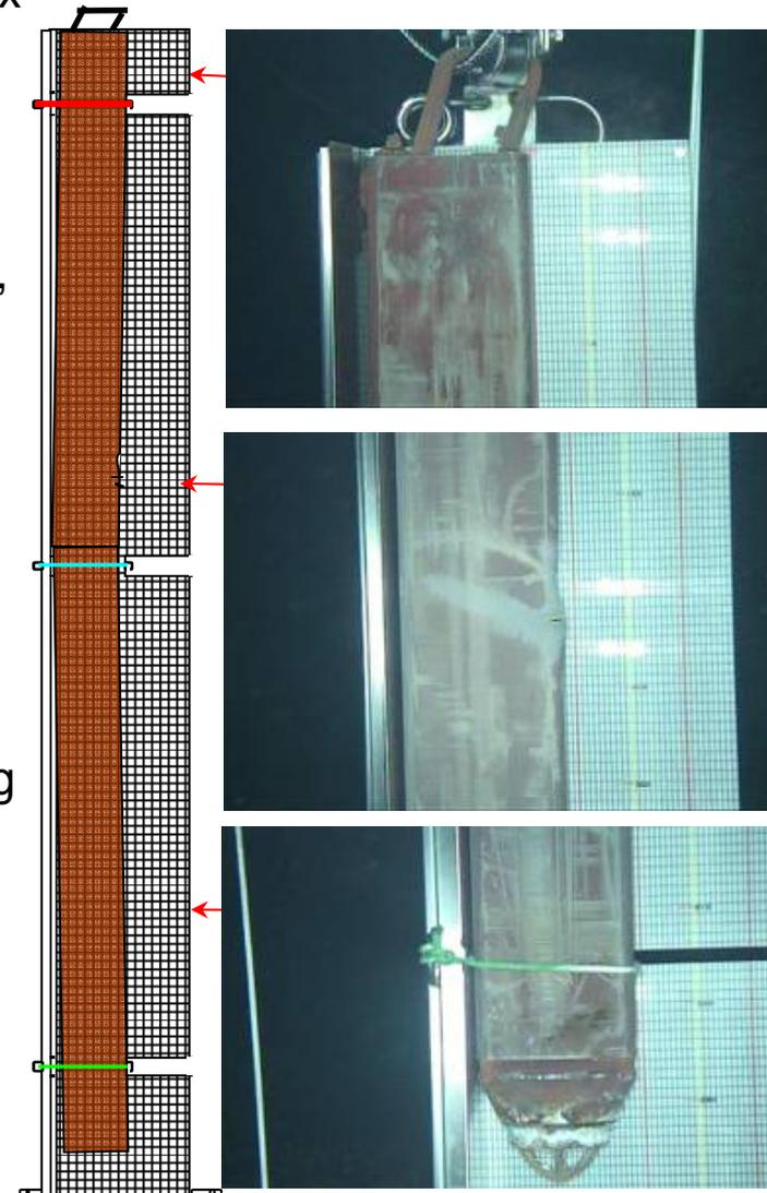
Measurement of the distortion degree of the deformed fuel
