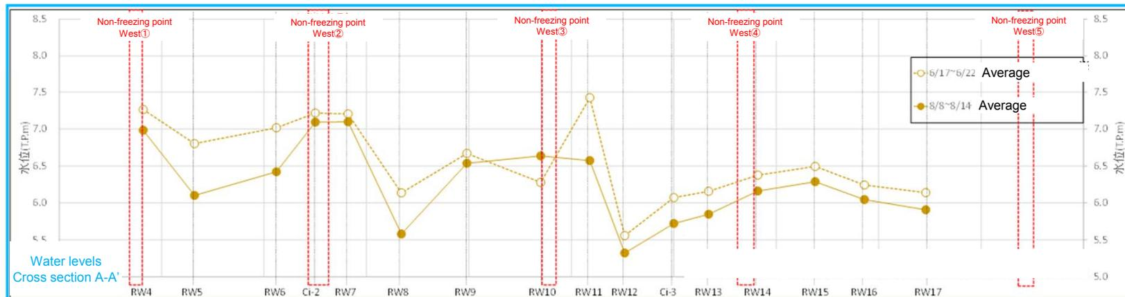
Water level distribution in the medium-grained sandstone layer inside the landside of the Landside Impermeable Wall
