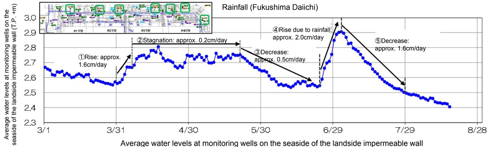
Average water levels at monitoring wells on the seaside of the landside impermeable wall
