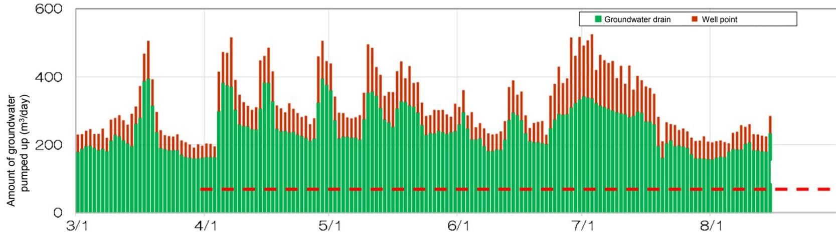
Amount of groundwater pumped up from the ground 4m above sea level (well points and groundwater drain)
