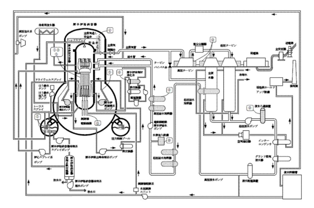
Schematic Flow Diagram of Fukushima Daiichi Unit 1
