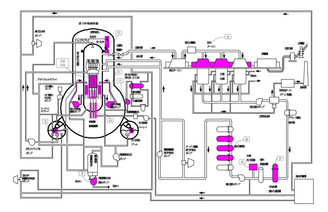
Schematic Flow Diagram of Fukushima Daiichi Unit 5
