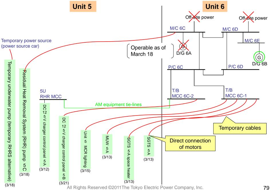
Fukushima Daiichi Unit 5 was restored and achieved cold shutdown by getting access to power from the emergency DG of Unit 6 and installing a temporary underwater pump to replace the RHRS pump of the sea water system.
