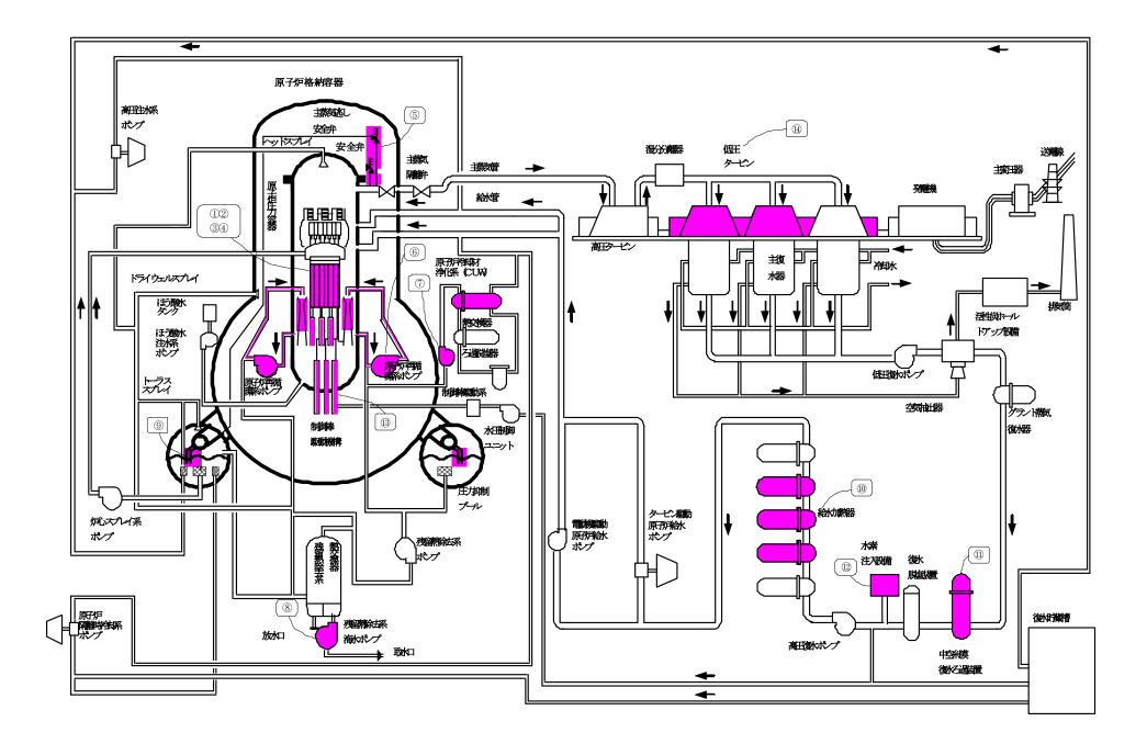
**Schematic Flow Diagram of Fukushima Daiichi Unit 3**
