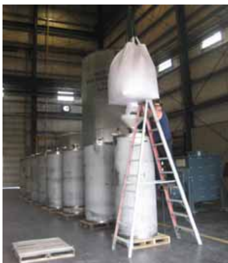
Filling of zeolite into vessel
