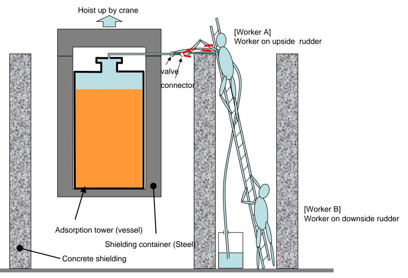
It should have been removed at "valve-close" though the hose had been removed at "valve-open", that caused water spewing out from connecting part and got the worker wet.
