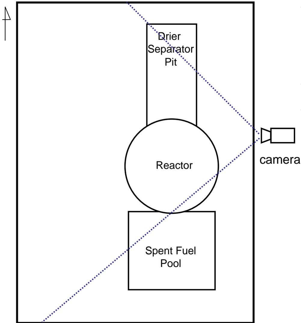
Layout drawing of 5<sup>th</sup> floor of Unit 2 reactor building in Fukushima Daiichi Nuclear Power Station
