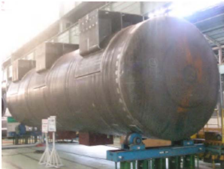
Iron storage tank for sludge in progress (External appearance)
