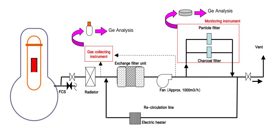
By switching flow path, either particle filter or Charcoal filter can be used for collection.
