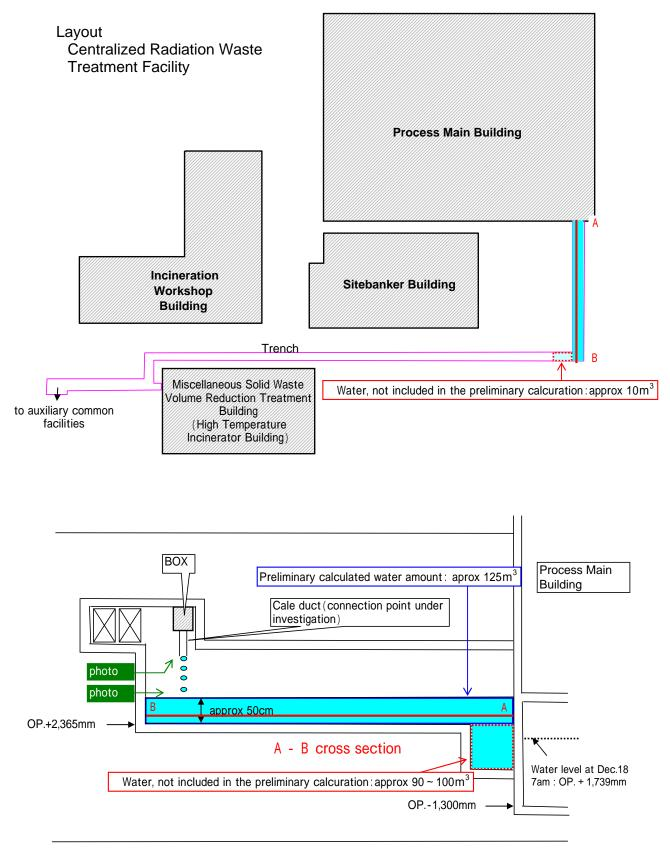
Accumulated water in the trench between Process Main Building and Miscellaneous Solid Waste Volume Reduction Treatment Building (High Temperature Incinerator Building) in the Centralized Radiation Waste Treatment Facility at Fukushima Daiichi Nuclear Power Station
