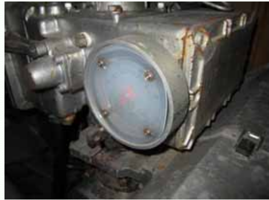
Distortion of Acrylic Plate on Valve Opening Indicator ( February 20, 2012 )
