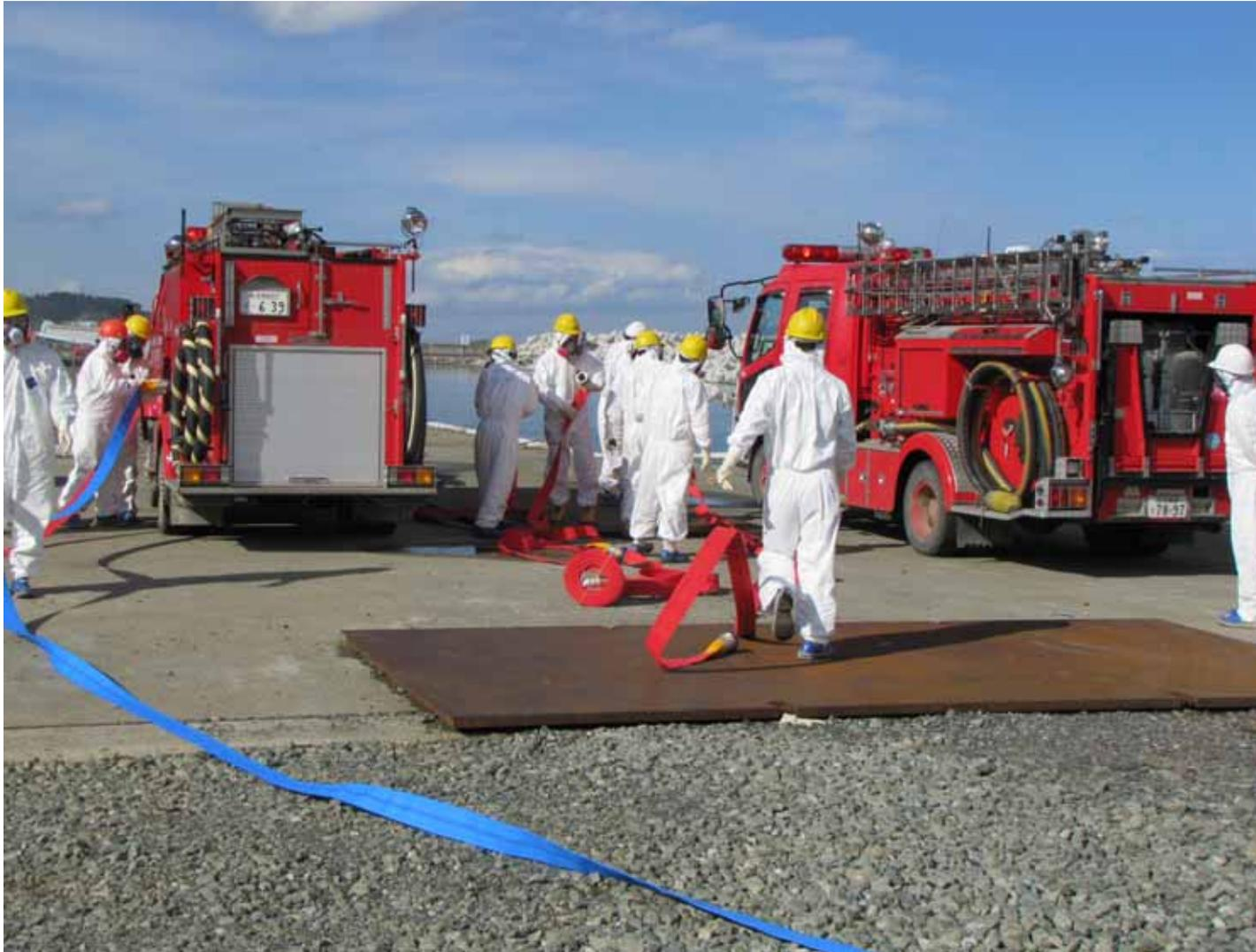
**Water injection to the reactor by using pump of fire truck
