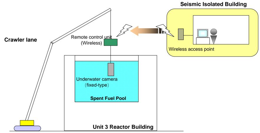
• The survey is conducted with a fixed-type underwater camera hung from the upper side of spend fuel pool using a crawler lane. The camera is operated by remote control unit from Seismic Isolated Building.
