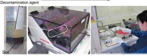
Cesium elution from soil using a shaker
