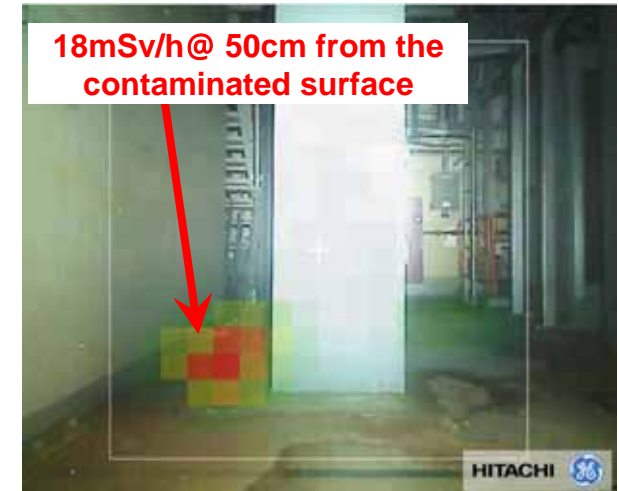
Image acquired at north side aisle after BG correction (Angle of elevation: 0 degree)
