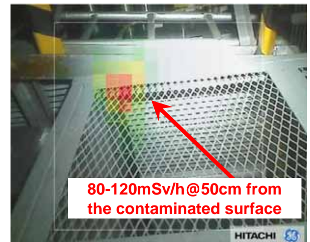
Image acquired at south side aisle after BG correction (Angle of elevation: 50 degree)
