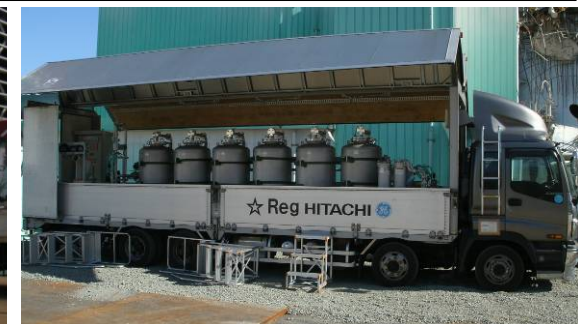
Ion exchanger used for desalting
