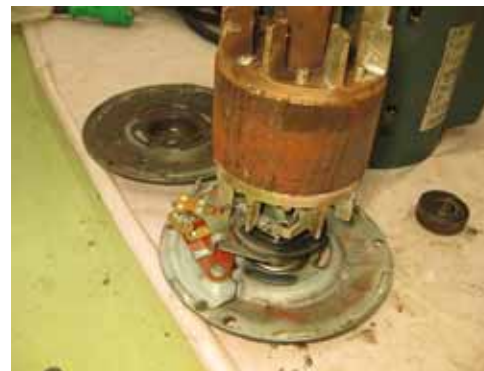
Inside the electric motor of H pump (rotor)
