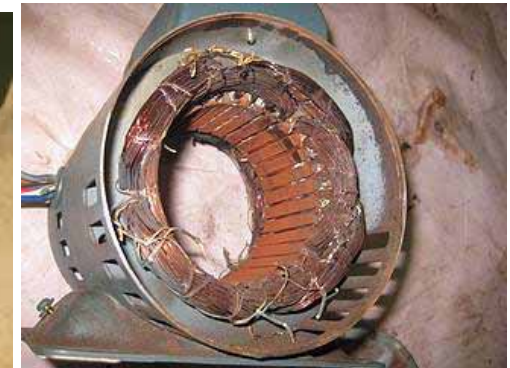
Inside the electric motor of H pump (stator)
