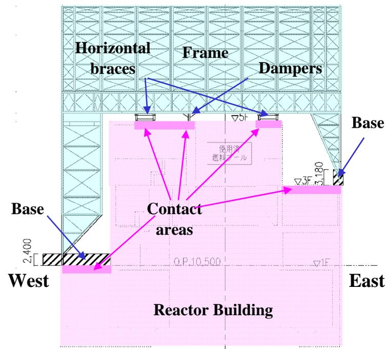
East-west cross section of the cover installed for fuel removal
