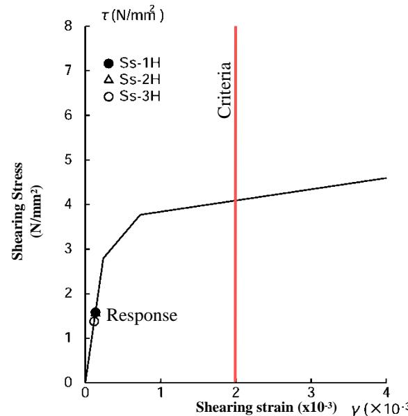
The maximum response on the shear skeleton of the earthquake-resisting walls
