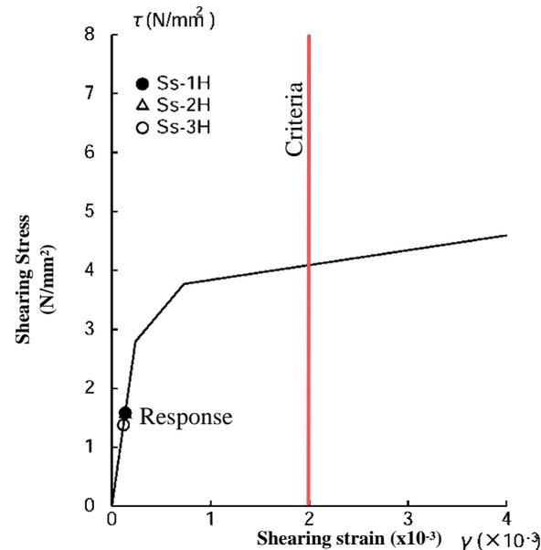
The maximum response on the shear skeleton of the earthquake-resisting walls of the auxiliary operation shared facility common pool building
