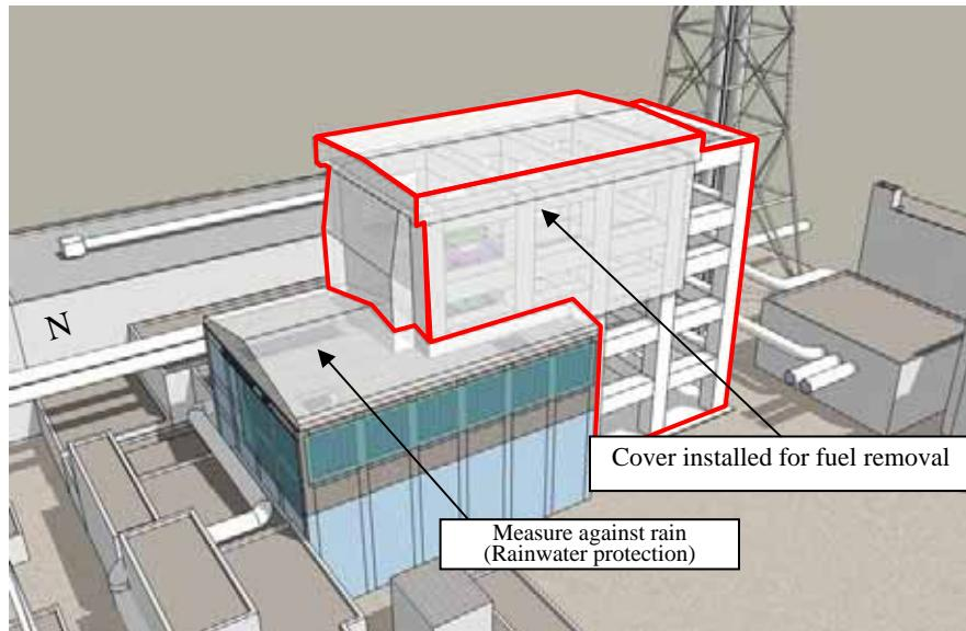
Cover installation for fuel removal at Unit 4 (Northwest side)
