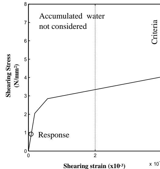
The maximum responses on the shear skeleton of Unit 1 Reactor Building basement walls in consideration of the accumulated water in the basement
