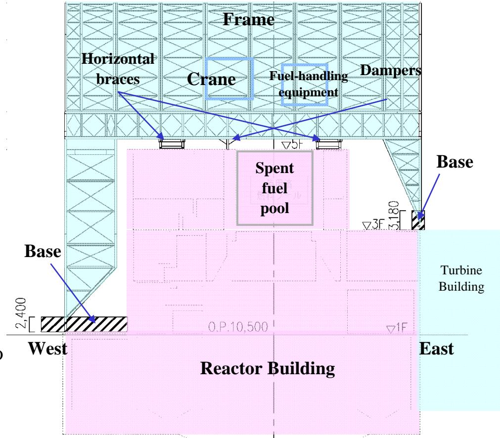
East-west cross section of the cover installed for fuel removal
