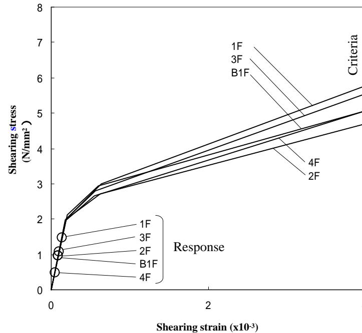
The maximum response on the shearing skeleton of the Reactor Building
