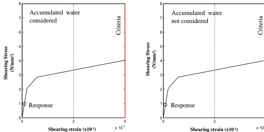
The maximum responses on the shear skeleton of Unit 1 Reactor Building basement walls in consideration of the accumulated water in the basement
