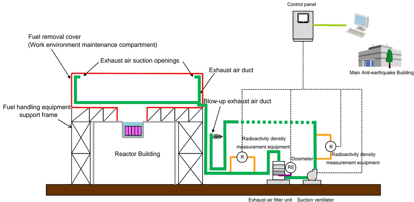
Overview of the ventilating equipment of the cover installed for fuel removal
