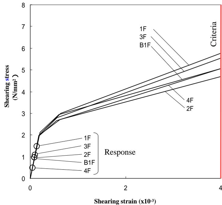
The maximum response on the shearing skeleton of the Reactor Building earthquake-resisting walls after cover installation
