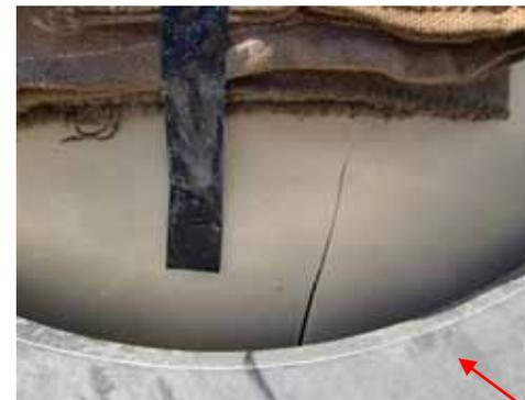
\* Damage found on the area with shape inconsistency.
