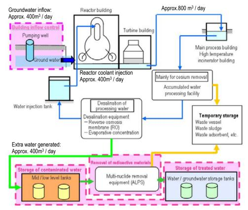
Figure 3: Overview of the accumulated water treatment
