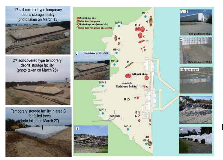
Figure 8: Dose reduction measures for debris and felled trees
