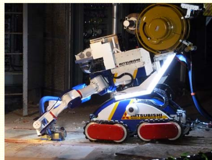
<Vacuuming and blast decontamination equipment>
