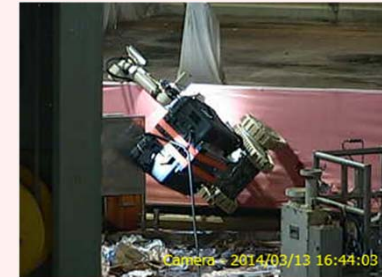
Status of remote-control robot falling down
