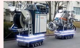
Dry ice blast decontamination equipment
