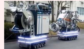
Dry ice blast decontamination equipment
