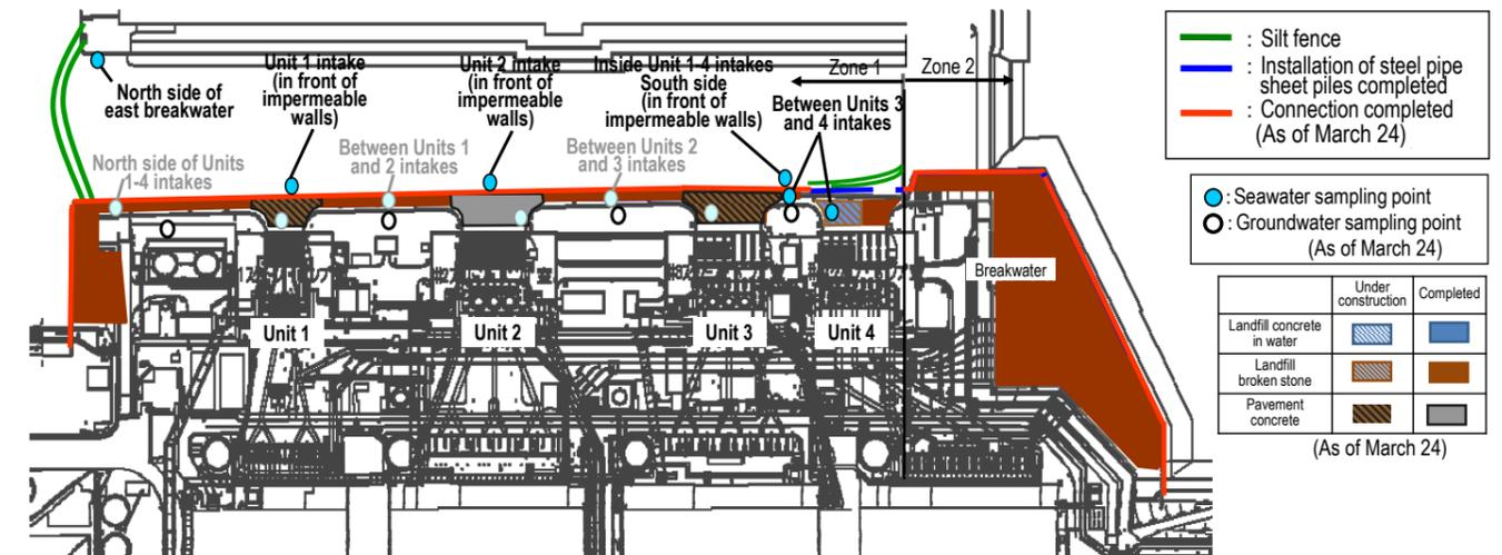
Figure 6: Progress status of impermeable walls on the sea side
