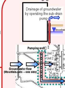
Aiming to reduce the level of groundwater by pumping subdrain water, tests were conducted to verify the stable operation of water treatment facilities, including subdrain.
