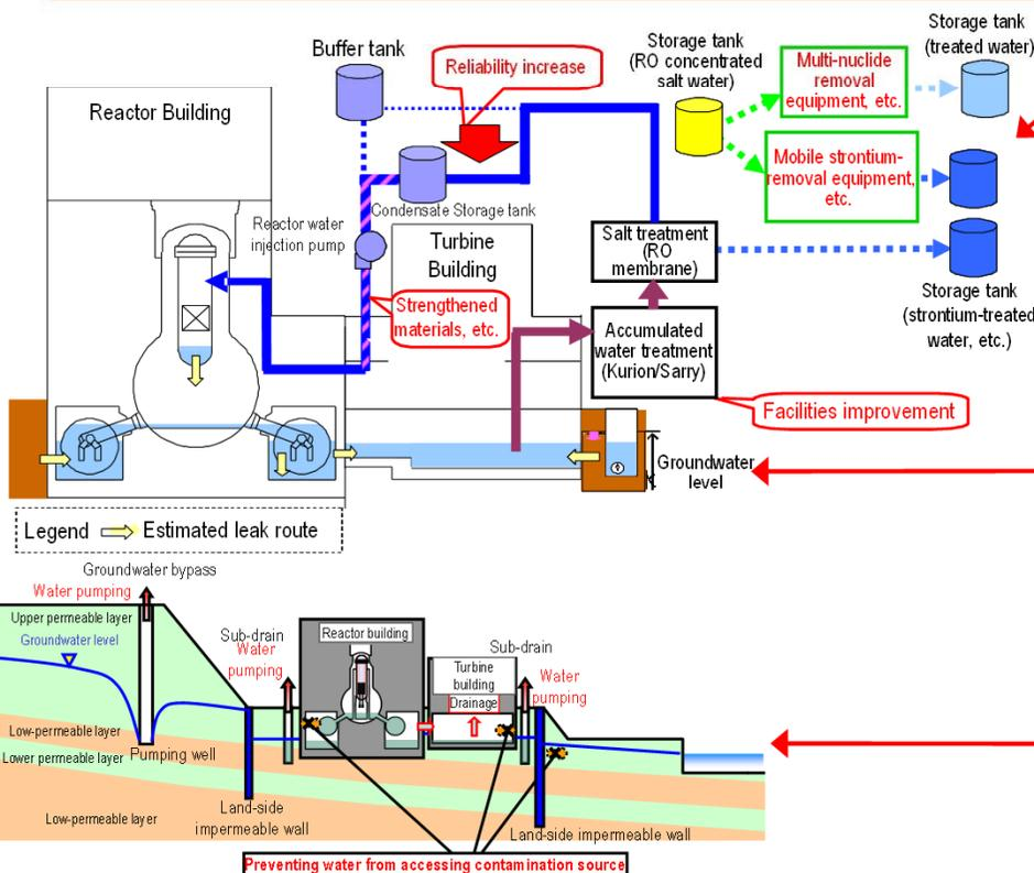
Preventing groundwater from flowing into the Reactor Buildings
