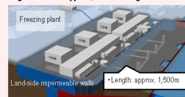
To prevent the inflow of groundwater into the Reactor Buildings, installation of impermeable walls on the land side is planned.
