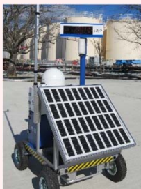
Installation of Dose-rate monitor
