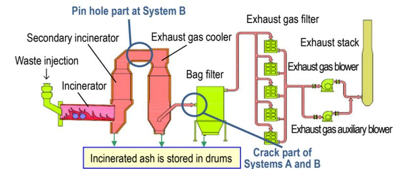
Figure 4: Overview of Radioactive Waste Incinerator
