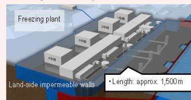
To prevent the inflow of groundwater into the Reactor Buildings, installation of impermeable walls on the land side is planned. Installation of frozen pipes commenced on June 2, 2014. Construction for freezing facilities was completed in February 2016. Freezing started on the sea side and at a part of the mountain side from March 2016 and at 95% of the mountain side from June 2016.
