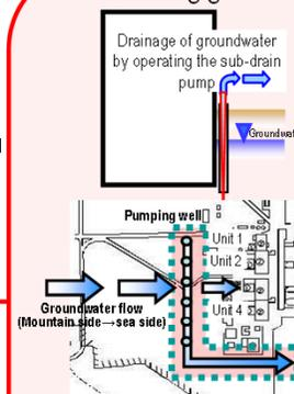
**Reducing groundwater inflow by pumping sub-drain water**
