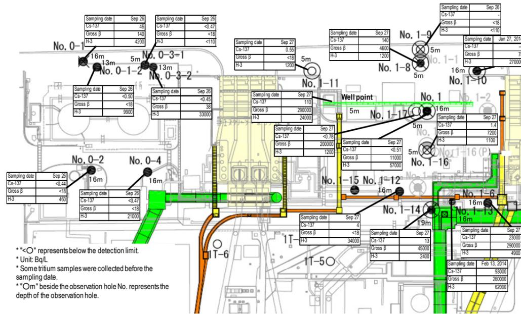
Figure 5: Groundwater density on the Turbine Building east side
