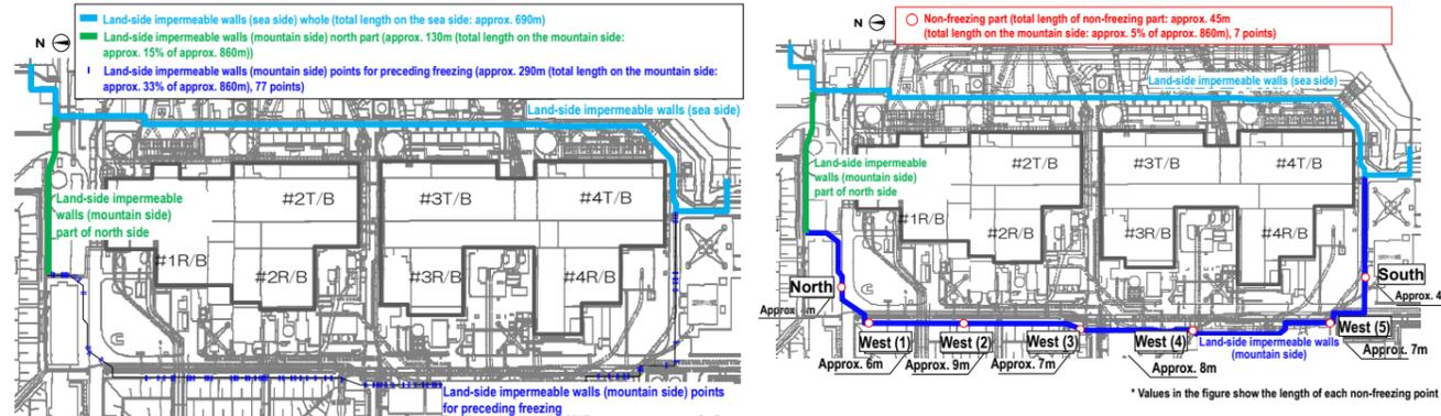
Figure 2: Scope of freezing of land-side impermeable walls
