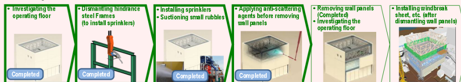
Flow of building cover dismantling
