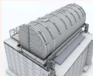
Image of the cover for fuel removal
