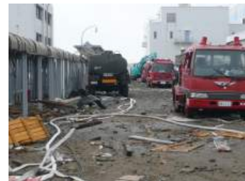
Injection by Fire Engine
