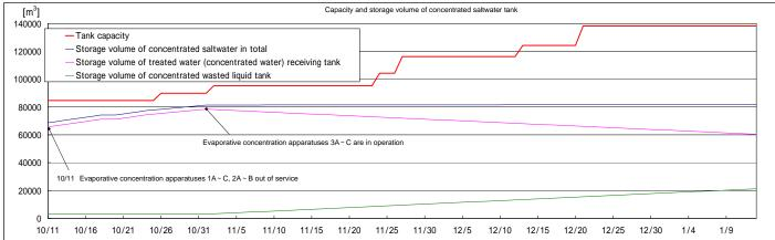
Note - Amount of water treatment is assumed to be 1,320m3/d (It can be adjusted according to level of accumulated water in T/B.)
