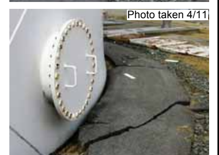
• Deformation due to collapse of tank lower area
