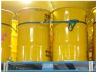
Drums secured with belts
