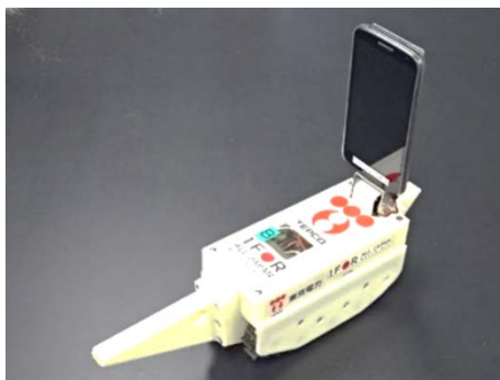
Robot used to survey the opening of the reactor containment vessel Installation of filtered venting equipment (Kashiwazaki-Kariwa Unit 7)
