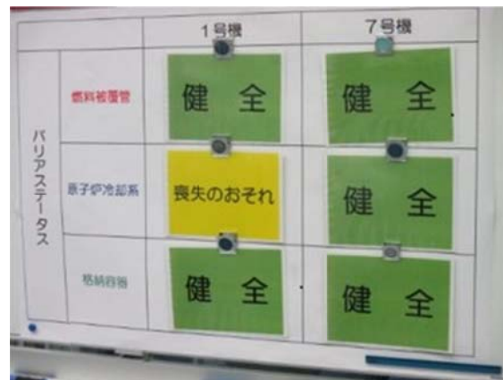
Good practices reflected in operations (barrier status board)
