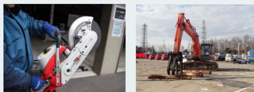
Example of a best proposal made a reality: "Deployment of heavy equipment used to remove debris left in the wake of a tsunami: Engine-powered cutter (left) (Fukushima Daini) and Claw-equipped excavator (right) (Kashiwazaki-Kariwa)
