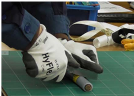
High voltage cable splicing training (Left: Cable cutting/shield removal, Left: Splicing)
