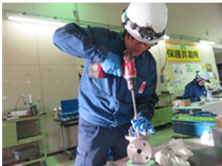
Valve disassembly inspection training (valve seat lapping)
