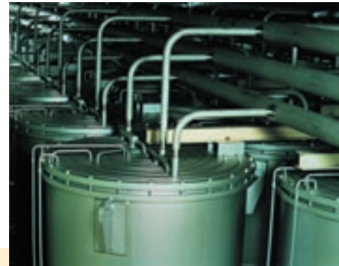
Uranium enrichment by the centrifuge process (Enrichment Plant of Japan Nuclear Fuel Limited)
