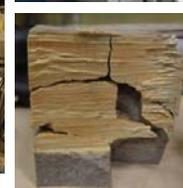
Fig 2 100mm cut on Zirconia under 5m of water
