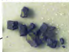
Upper core debris bed
