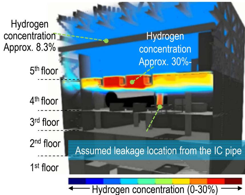
Figure 1: Distribution of hydrogen immediately before the explosion
