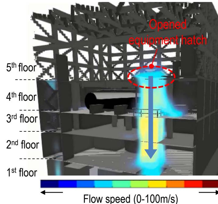
Figure 2: Distribution of blast speed (after the equipment hatch lid was opened)
