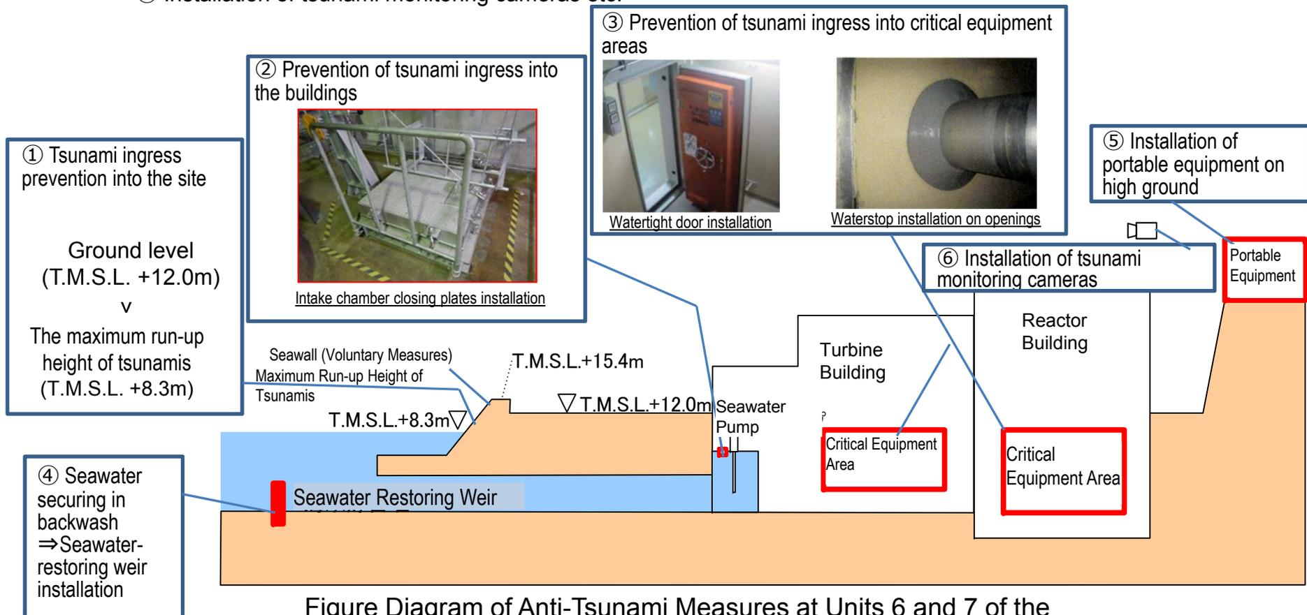
Figure Diagram of Anti-Tsunami Measures at Units 6 and 7 of the Kashiwazaki-Kariwa Nuclear Power Plant
