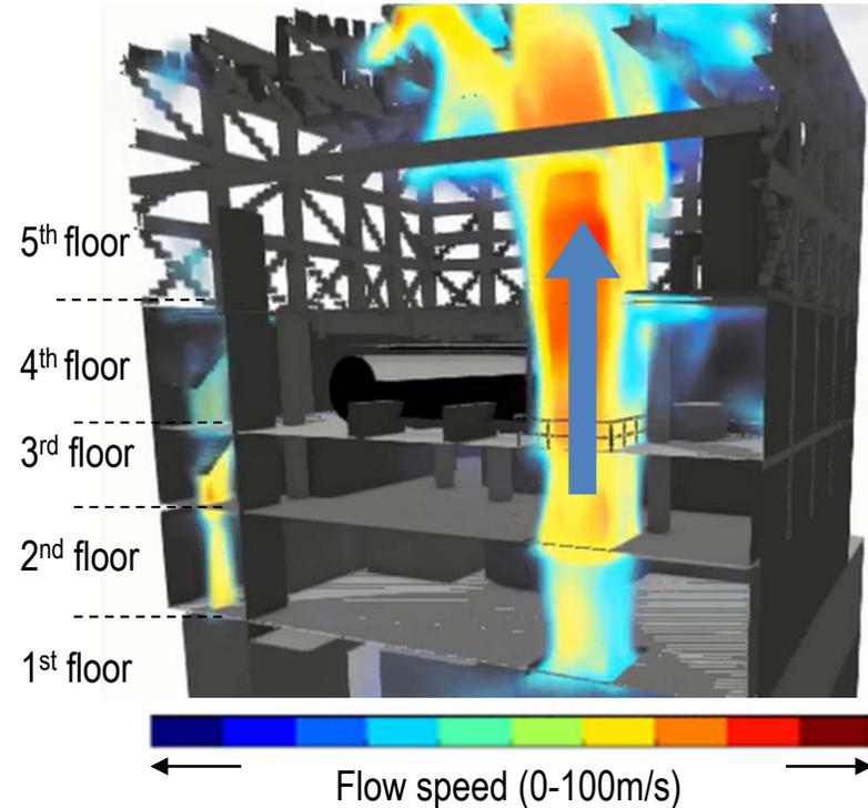
Figure 2: Distribution of blast speed (after the 5<sup>th</sup> floor side wall was damaged)
