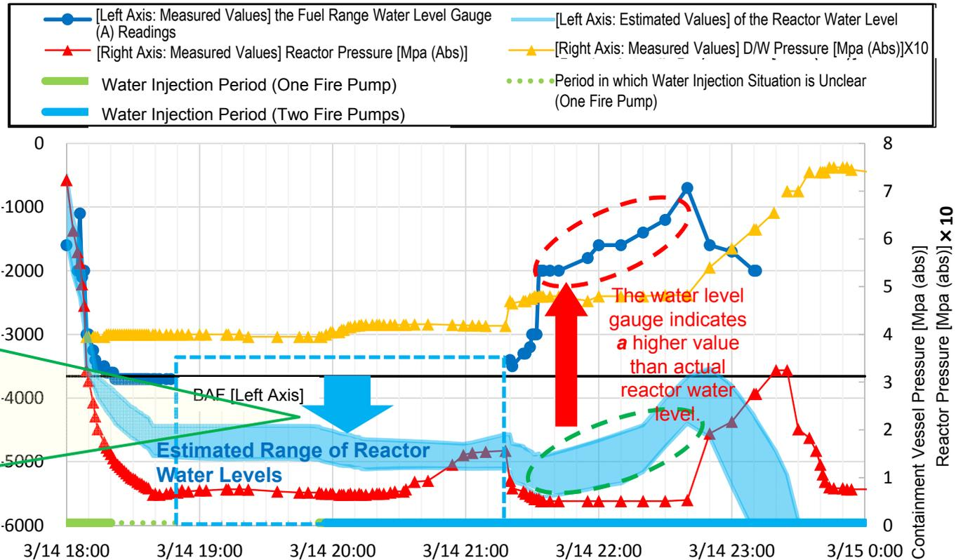
We evaluated the reactor water level ranges from 18:00 to around 22:40 on March 14, which corresponds to the period of progressive core damage and meltdown as follows\*:
