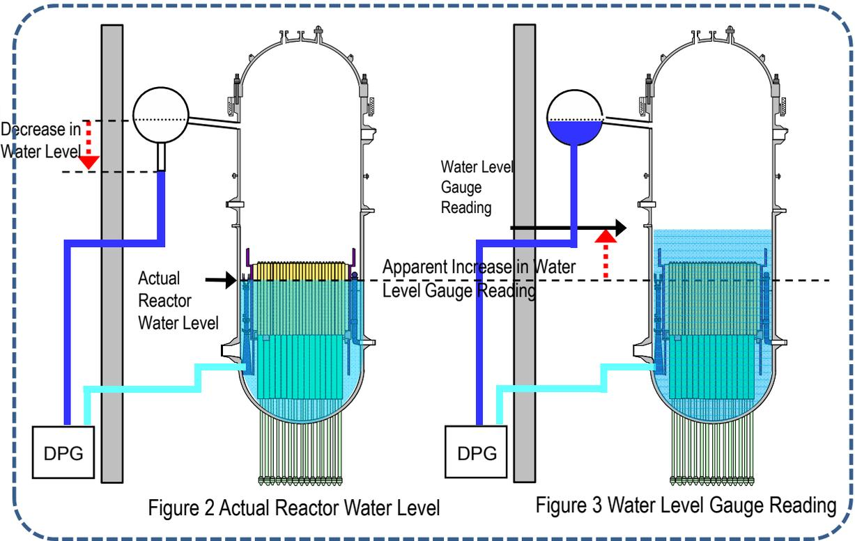
Figure 2 Actual Reactor Water Level
