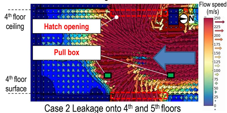
The distortion direction of the pull boxes around the 4<sup>th</sup> floor equipment hatch was consistent with the direction of the blast in the case of leakage onto the 5<sup>th</sup> floor. The blast direction in the case of leakage onto the 4<sup>th</sup> and 5<sup>th</sup> floors differed from the distortion direction of the pull boxes.
