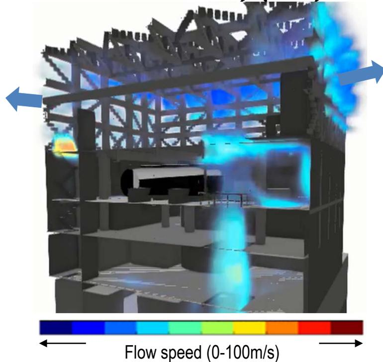
Figure 1: Distribution of blast speed (when the 5<sup>th</sup> floor wall side was damaged)
