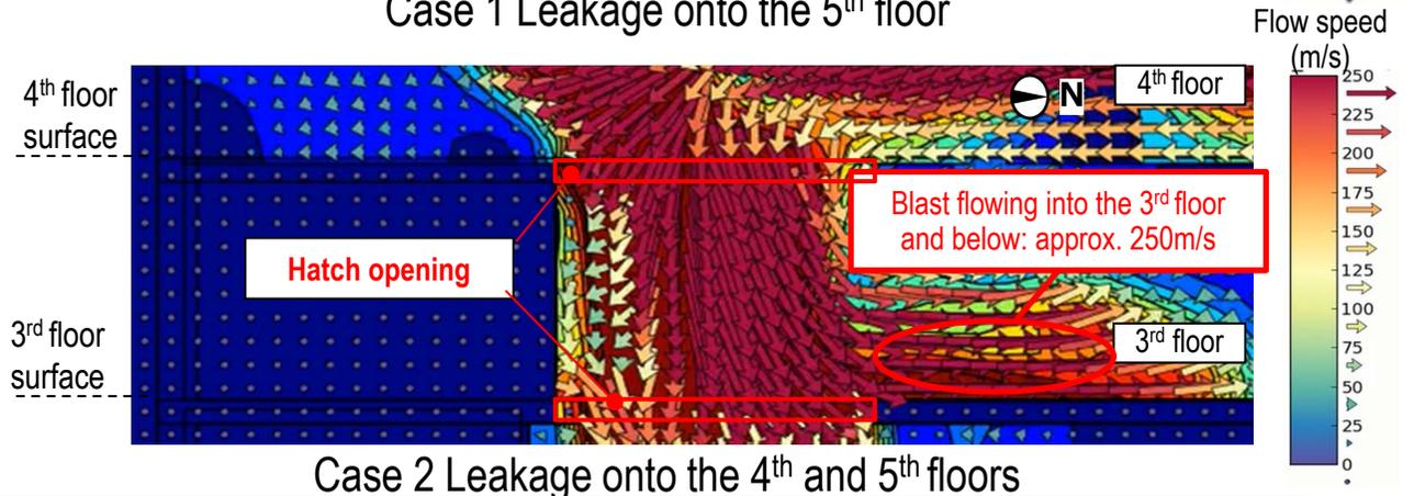
Minor damage was identified on the 3<sup>rd</sup> floor and below and in terms of the inflow blast speed, it was consistent with the case of leakage onto the 5<sup>th</sup> floor. The blast in the case of leakage onto the 4<sup>th</sup> and 5<sup>th</sup> floors was likely to be excessive.
