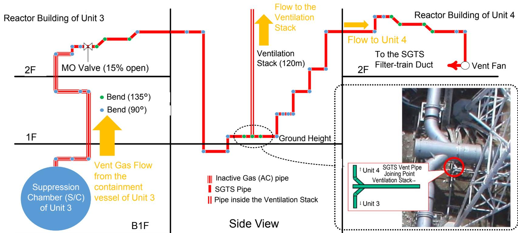
Figure Diagram of Vent Pipes and SGTS Pipes
