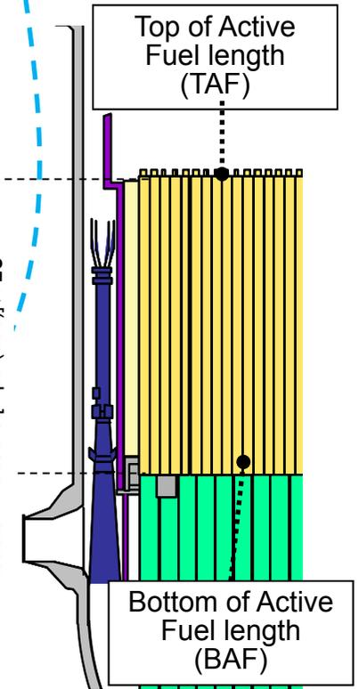
\* The reactor water level decreased to BAF or below due to the decompression of the reactor.
