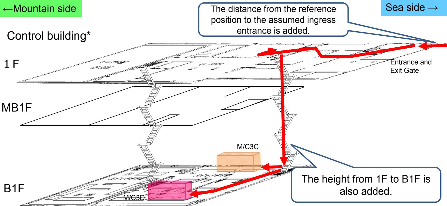
Figure Assumed Main Tsunami Intrusion Paths to M/C3C and 3D of Unit 3.
