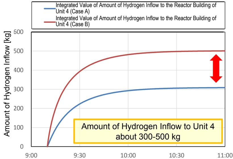
Figure 1 Amount of Hydrogen which Flowed into the Reactor Building of Unit 4
