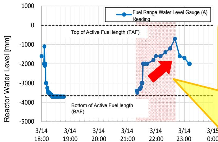
Figure Water Level Gauge Readings of Unit 2
