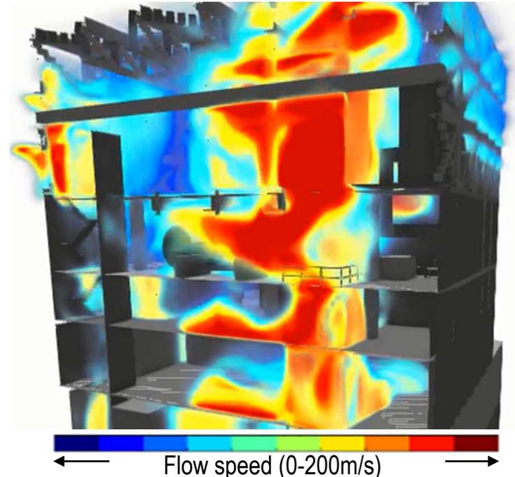
Figure 2: Distribution of the blast speed (when the 5<sup>th</sup> floor side wall was damaged)
