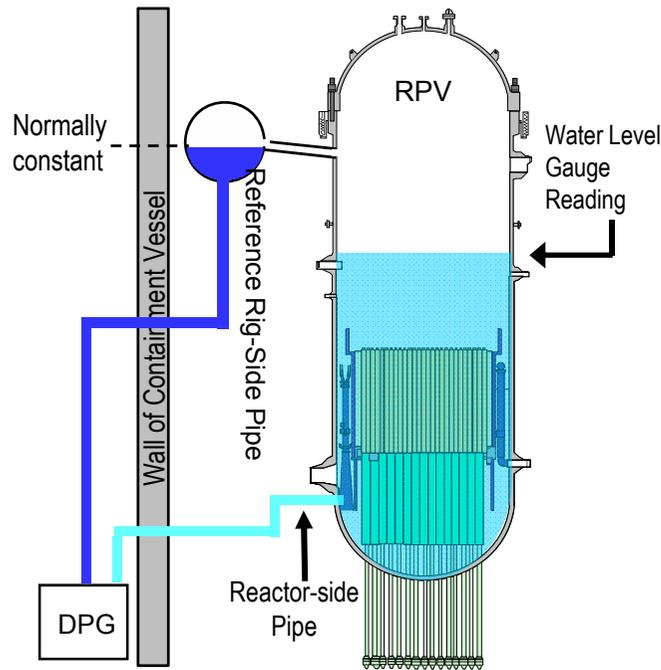
Figure 1 Structures of the Water Level Gauge
