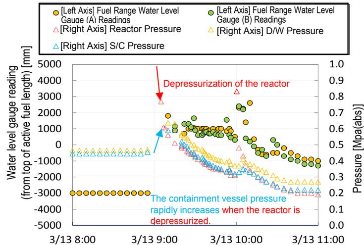
Figure 1 Parameters at the Start of Containment Vessel Vending
