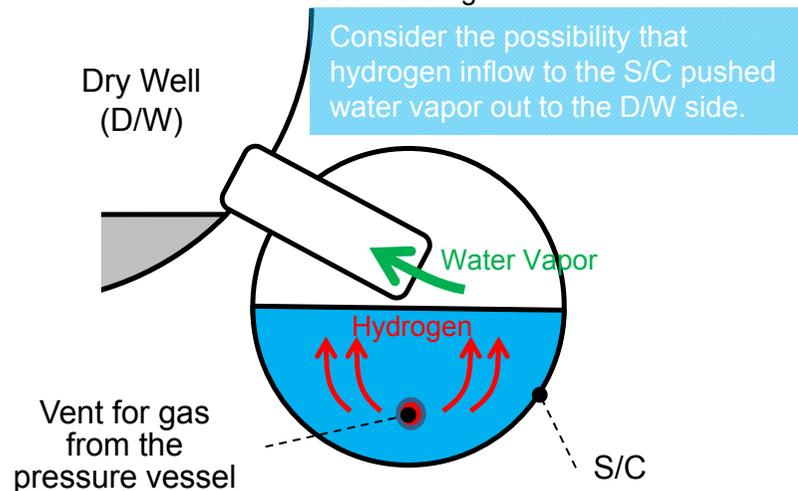
Figure 2 Vapor behavior in the S/C in hydrogen inflow
