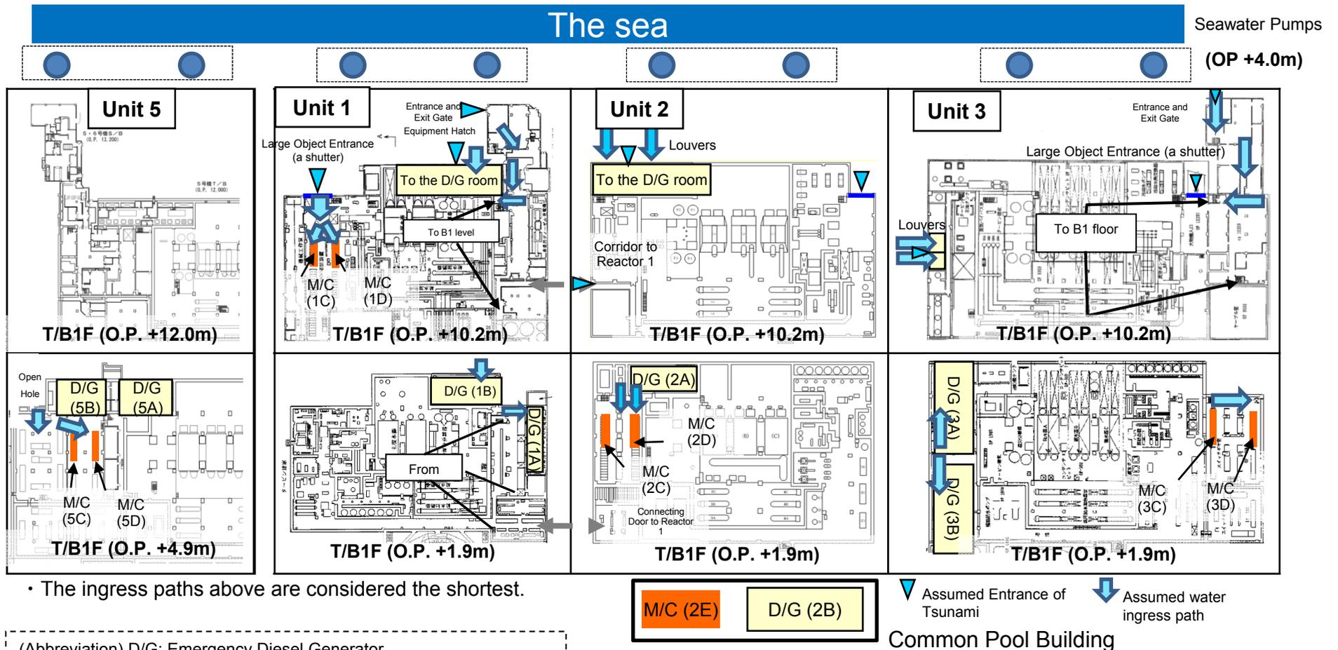
Figure Main Intrusion Path to Each Unit
