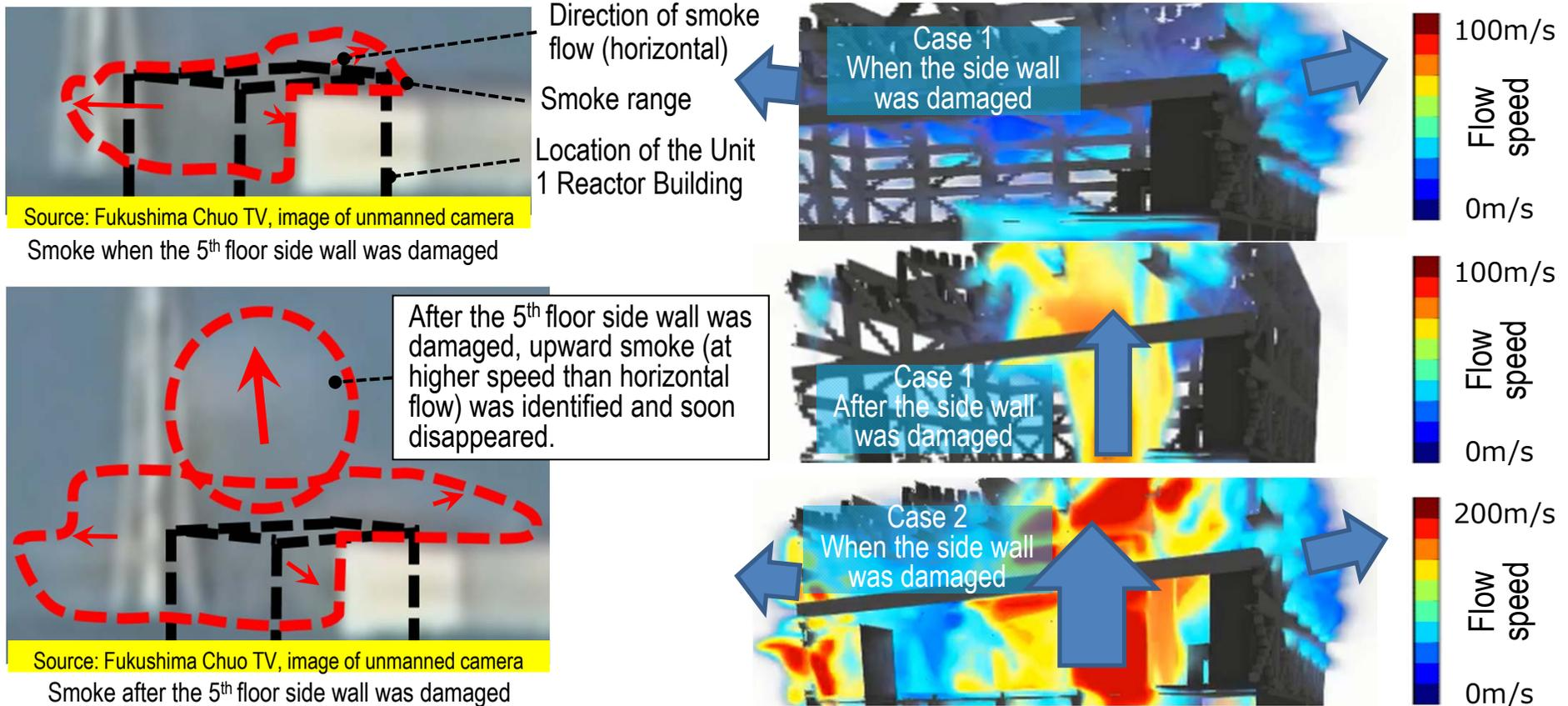
The images captured the potential upward flow after the side wall was broken, which was indicated in the case of the leakage on the 5<sup>th</sup> floor.
