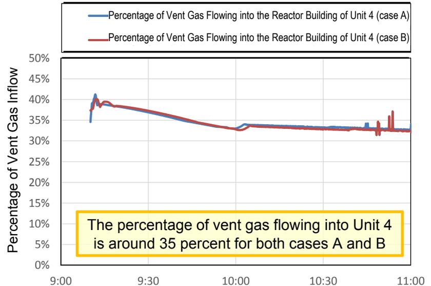
Figure 2 Percentage of vent gas flowing into the reactor building of Unit 4
