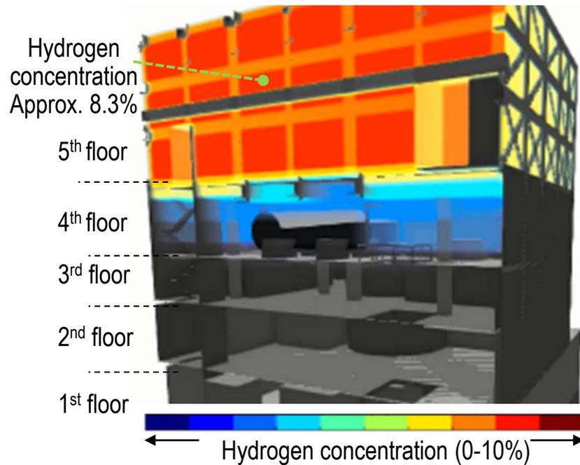
Figure 1: Distribution of hydrogen concentration immediately before explosion
