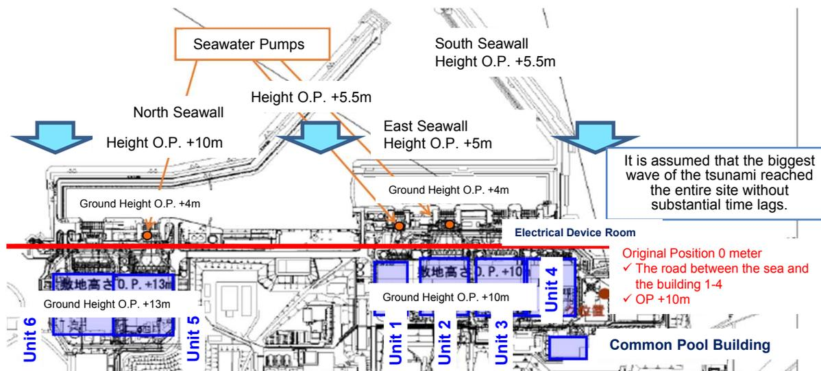
Figure Assumption of Each Reactor Building, the Location of the Seawater Pump, and Tsunami Runup
