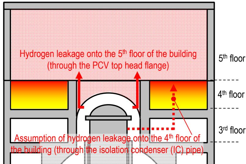
Figure: Image of hydrogen leakage route to the Reactor Building
