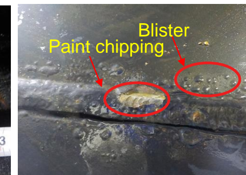
Scratches, etc., found at the bottom of the tank
