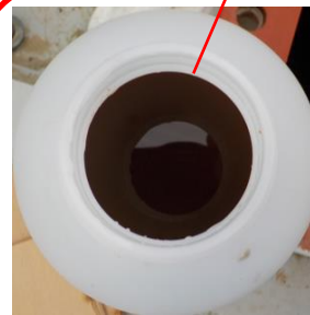
External appearance of water at the bottom of the RO concentrated water receiving tank sampled on February 19, 2019
