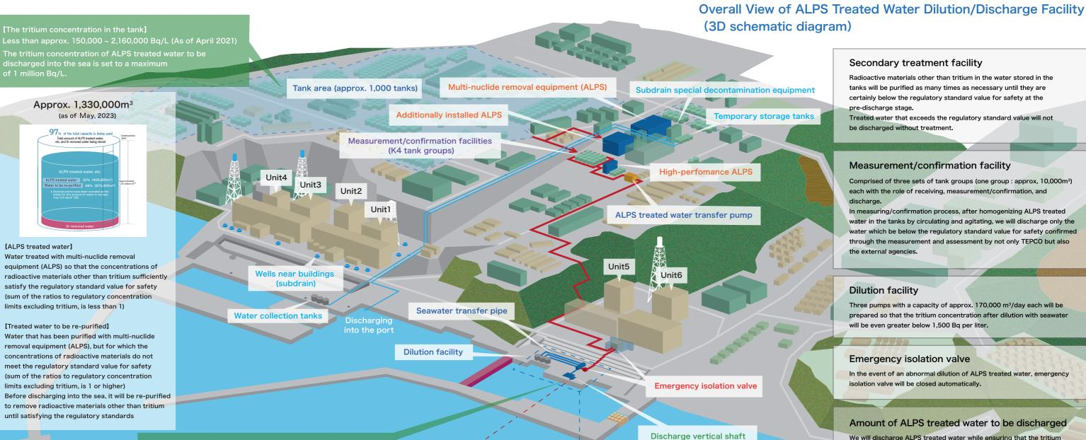
[The tritium concentration inside the discharge vertical shaft] Less than 1,500 Bg/L
