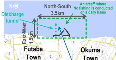
The outlet of the discharge tunnel is installed within the area\* where no fishing is conducted on a daily basis, and the assumed quantity of water within the subject area is approx. 60 billion liters.
